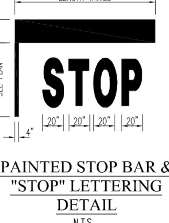
PAINTED STOP BAR & "STOP" LETTERING N.T.S.
